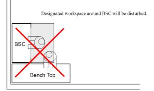
Biological Safety Cabinet (BSC) performance can be impacted by airflow patterns in the room, especially at the face of the cabinet. To ensure this does not happen, follow the guidelines listed below:
